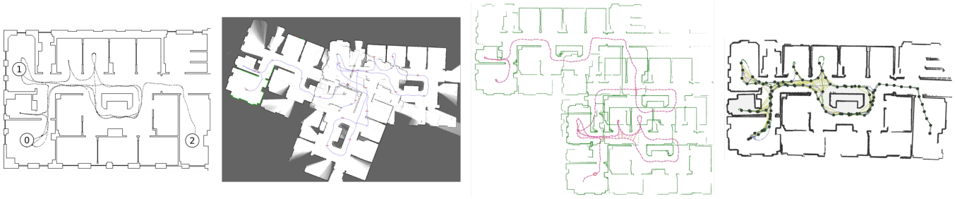
Fig. 10: From left to right: Simulated ground truth map with exploration path, map generated by Cartographer, map generated by SRRG mapper 2D, map generated by our system. Albeit the individual components of our system are rather standard, it can cope with unforeseen events thanks to the proposed SLAM state machine.
